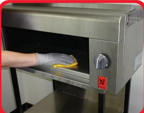
**Step 2 - Using all purpose cleaner and a cloth clean the inside and outside surfaces of the grill.**
