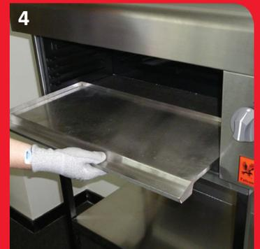
**Step 1 - Remove aluminium brander (1), upper drip tray (2), wire shelf (3) and base drip tray (4) and wash in hot soapy water. A non abrasive scourer may be used to remove stubborn stains. Leave to soak if necessary. Rinse and dry.**
